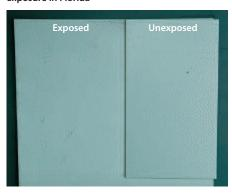
A year's exposure to sunlight in Florida can equate to four to seven years of exposure in Northern Europe. Based on the test results to date, Colorcoat HPS200 Ultra® has had UV exposure equivalent to up to 21 years exposure in Northern Europe with excellent gloss and colour retention.
