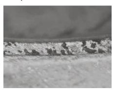
Figures 8 and 9 illustrate how, as the lighter coloured Zinc dendrites ultimately corrode, the unique microstructure of the Galvalloy® layer ensures that the surface coating remains adhered to the eutectic surface.
