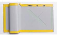
Colorcoat HPS200 Ultra® showed minimal (less than 3mm) edge and scribe delamination following repeated cycles of testing.
