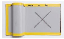
Figure 22. Test panel after Watersoak 1000 hours
