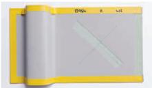
excellent paint adhesion between the Galvalloy® metallic coating and the organic layers of Colorcoat HPS200 Ultra®. In figures 21, 22 and table 4 the topcoat has been removed to clearly show absolutely no creep at the scribe, or cut edge.
