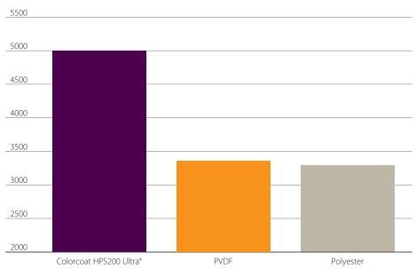
Figure 11. Abrasion resistance comparison (ASTM D968:2001)
