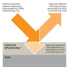
All colours in the Colorcoat HPS200 Ultra® range have been tested to determine their reflectivity performance. The heat absorption and emittance values for each colour have also been measured, along with the maximum surface temperature for the various colours under standard conditions. The total solar reflectance (TSR) was measured according to ASTM E903-96 and emissivity according to ASTM C1371-04a.
