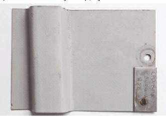
Figure 18. Colorcoat HP200® 18 years exposure at coastal weathering site at Rye, England.
