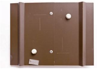
Figure 17. Colorcoat HPS200° with Galvalloy° metallic coating – 13 years exposure at coastal weathering site at Rye, England.
