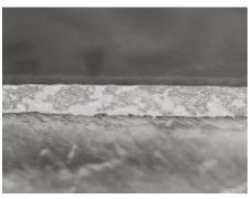
Figure 9. Galvalloy® microstructure after corrosion
