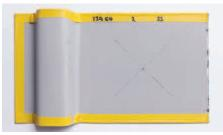
Figure 21. Test panel after humidity 1000 hours
